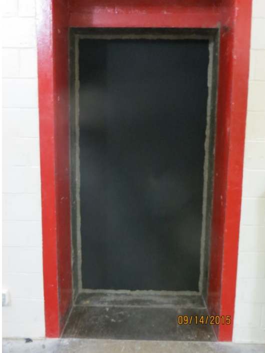
Figure 1 – Specimen mounted in the test opening (source side).
