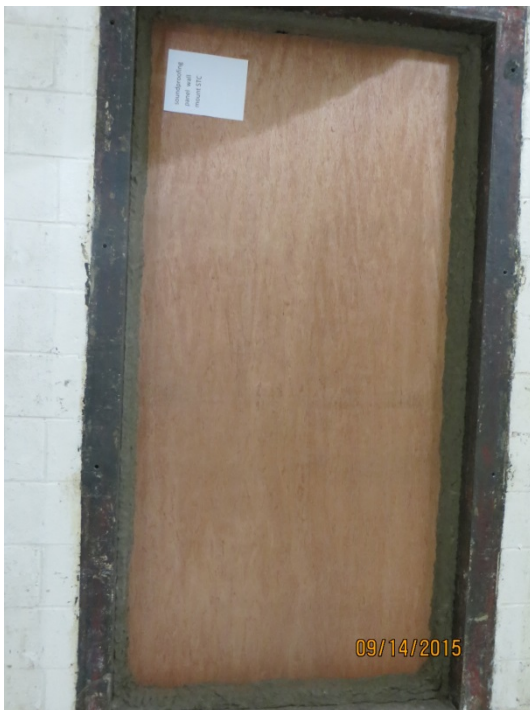
Figure 2 – Specimen mounted in the test opening (receive side).
